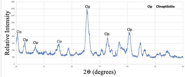
The XRD analysis data for the KMI clinoptilolite is displayed in the plot below:
